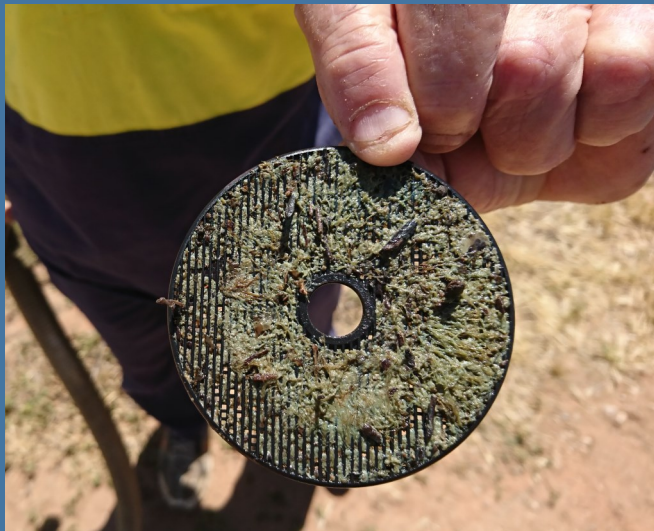
Bryozoa clogging a water meter filter
