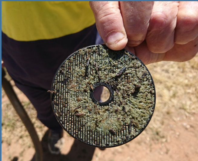
Bryozoa clogging a water meter filter
